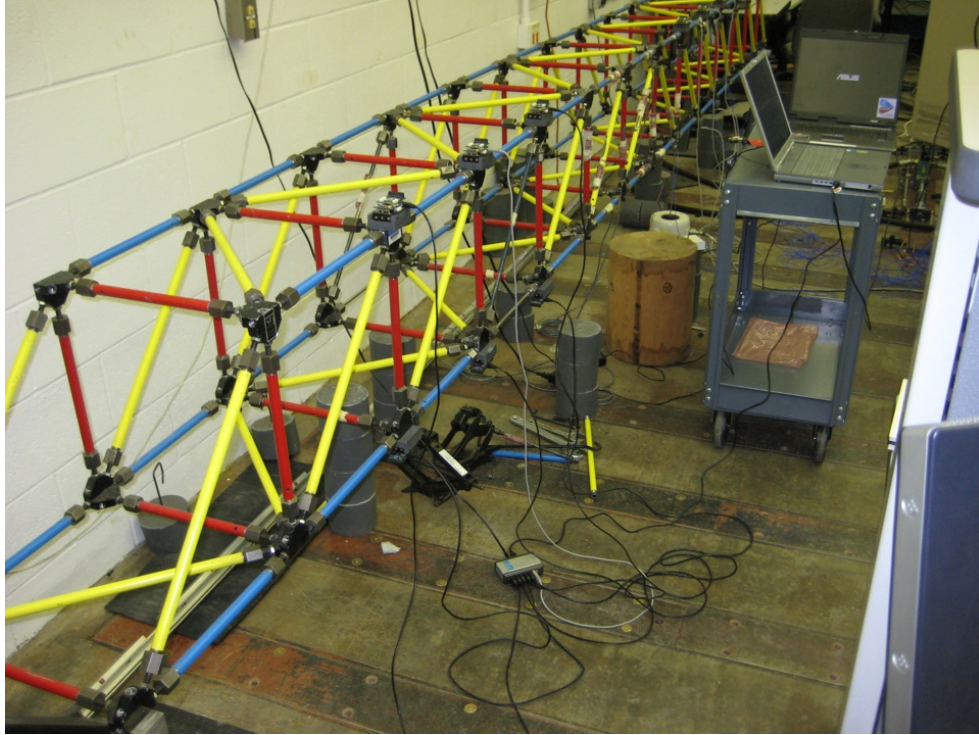
Figure 3.9: 3D truss test structure
